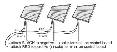
Attach BLACK to negative (–) solar terminal on control board attach RED to positive (+) solar terminal on control board.
